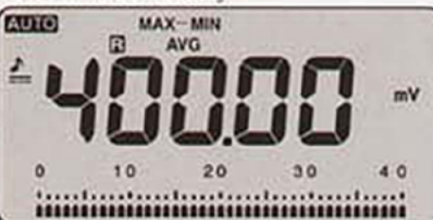
Fig 6: RECORD Function Display
