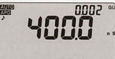
Fig 5: nS + G \Omega Display
