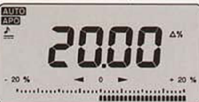
Fig 3: RELATIVE % CHANGE Display
