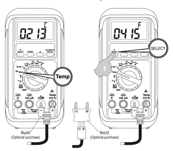
Note: Be sure to insert the banana plug type-K temperature bead probe Bkp60 with correct + — polarities. You can also use a plug adapter Bkb32 (Optional purchase) with banana pins to type-K socket to adapt other standard type-K mini plug temperature probes.
