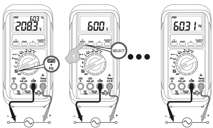
Function defaults at **VFD-ACV** \*Hz. By default, voltage is set at 600V & 1000V two auto-ranges to best cope with most Variable Frequency Drives (VFD) measurements. High noise-rejection frequency measurement algorithm and Low-pass filter circuit are permanently bundled with all the voltage and frequency function-ranges within this rotary-switch position. Press the **RANGE** button momentarily to select other ranges only when needed.
