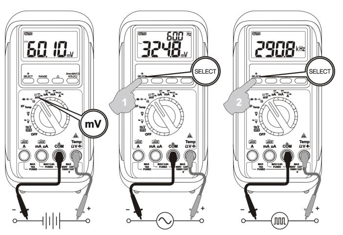
**DCV**Turn rotary switch to DCV function position directly.
