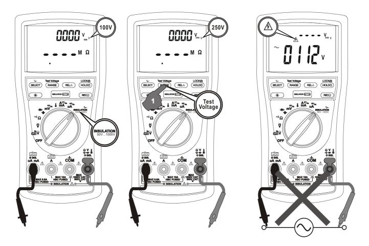
Default startup primary display reading is "-.---". Allow enough  $\boxed{\text{IEST}}$  time for a good measuring result. After the  $\boxed{\text{IEST}}$  is released, the measuring loop starts to discharge the testing voltage. The last measured resistance reading stays on the primary display until the next  $\boxed{\text{IEST}}$  or a function change. The secondary display keeps showing the actual detected voltage readings.
