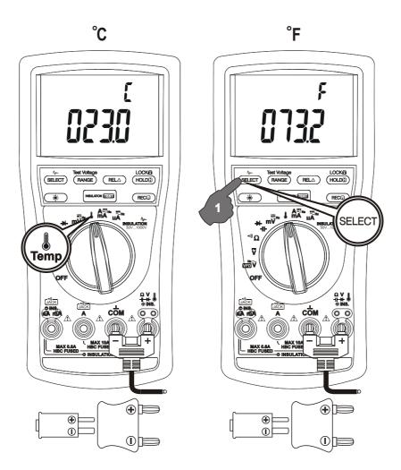
Note: Be sure to insert the banana plug type-K temperature bead probe Bkp60 with correct + – polarities. You can also use a plug adapter Bkb32 (Optional purchase) with banana pins to type-K socket to adapt other standard type-K mini plug temperature probes.
