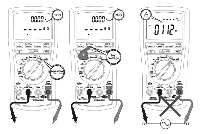
The  $\overrightarrow{\text{IEST}}$  is active as long as the **TEST** button is pressed and hold. The **TEST** buttons on the meter and on the Remote Probe work alike. The Insulation Resistance readings are shown on the primary display.
