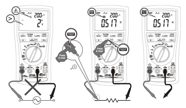
**Lock-Test mode** is recommended for continuous measurements. To apply, press the **LOCK** button momentarily to display the annunciator **DLOCK** before pressing the **TEST** button momentarily. The LCD will show both **DLOCK** & **TEST** to indicate continuous measurement is active. Press again either button momentarily to release the Lock-Test mode.
