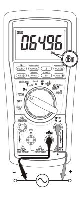
**Note:** In **dBm** function, power up default reference impedance will be displayed for 1 second before displaying the dBm readings. Press **dBm-\Omega** (**RANGE**) button momentary to select different reference impedance of 4, 8, 16, 32, 50, 75, 93, 110, 125,
