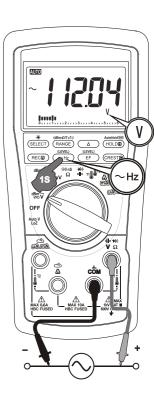
**Note:** It is recommended to direct measure the signals (voltage or current) in autoranging mode before activating the ~Hz function right in that range to get the most appropriate trigger level automatically. If the ~Hz reading is unstable, select lower sensitivity to avoid possible electrical noises. If the reading shows zero, select higher
