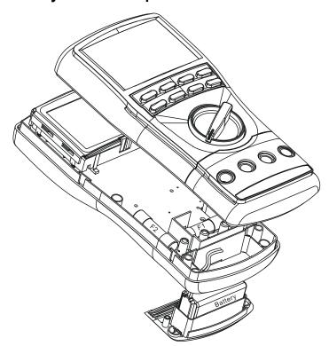
**Battery use:** Single 9V battery; NEDA1604G, JIS006P IEC6F22, NEDA1604A, JIS6AM6 or IEC6LF22
