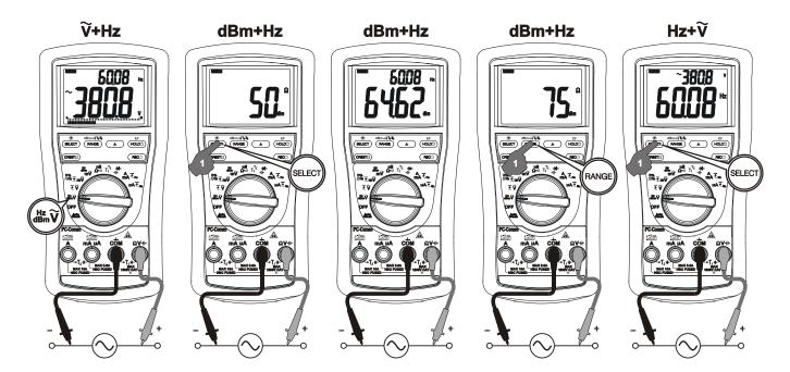
Note: Hz Input sensitivity varies automatically with voltage (current function alike) range selected. 1V range has the highest and the 1000V range has the lowest. Auto-ranging measurements normally set the most appropriate trigger level. You can also press the
