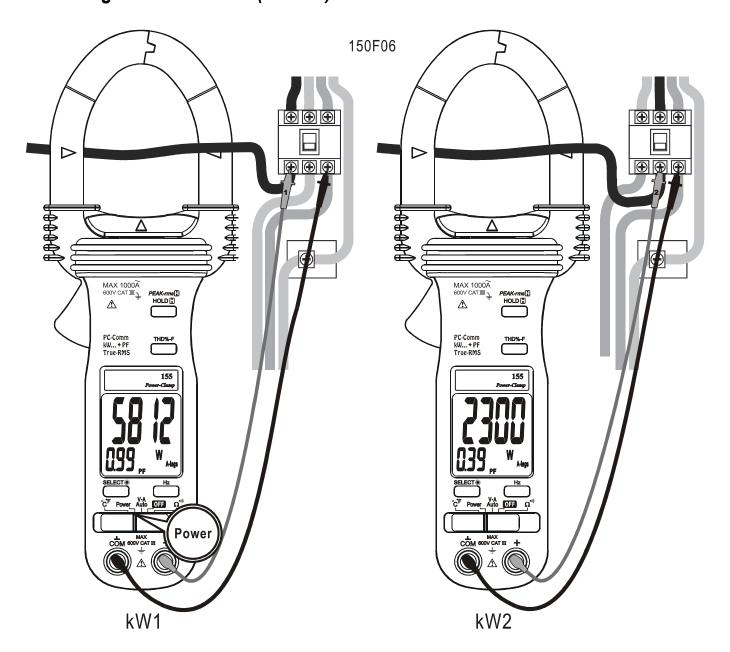
In both un-balanced and balanced load cases, 3-Phase 3-Wire ( $3\sim3W$ ) systems, measure the power components  $kW_1$  and  $kW_2$  separately as illustrated. System (total) power  $kW_{Total}$  is the summation of the two measured power components. That is:
