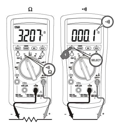
•)) BeepLit<sup>TM</sup> Continuity function is having improved convenience for checking wiring connections and operation of switches. A continuous beep tone together with flashing display backlight indicate a complete wire. Such audible and visible indications improve continuity readabilities in noisy working environments.
