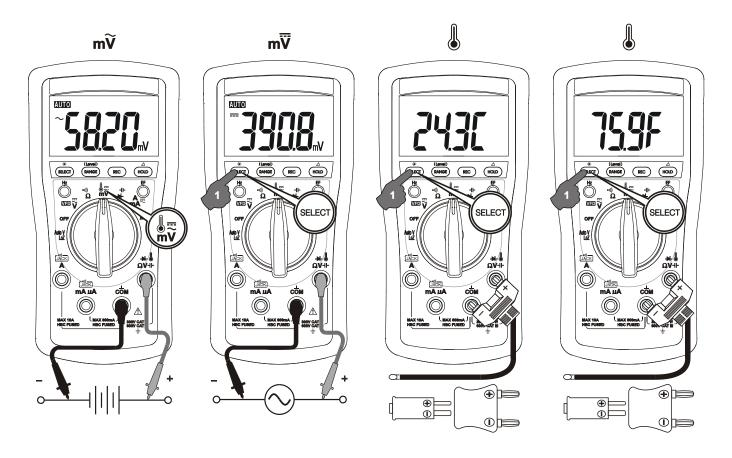
Note: Be sure to insert the banana plug type-K temperature bead probe Bkp60 with correct **+ -** polarities. You can also use a plug adapter Bkb32 (Optional purchase) with banana pins to type-K socket to adapt other standard type-K mini plug temperature probes.
