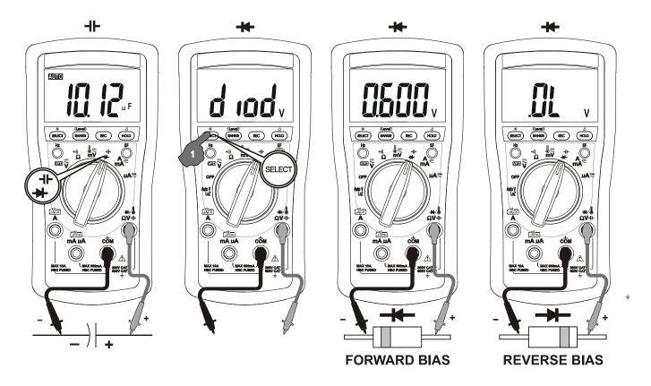
In **Diode** function, the normal forward voltage drop (forward biased) for a good silicon diode is between 0.400V to 0.900V. A reading higher than that indicates a leaky diode (defective). A zero reading indicates a shorted diode (defective). An OL indicates an open diode (defective). Reverse the test leads connections (reverse biased) across the diode. The digital display shows OL if the diode is good. Any other readings indicate the diode is resistive or shorted (defective).
