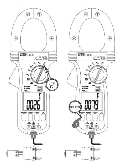
Defaults at °C (Celsius) readings. Press **SELECT** button momentarily and release to select °F (Fahrenheit) readings. Inputs are made through the test lead terminals. Be sure to insert the banana plug type-K temperature bead probe Bkp60 with correct + – polarities. You can also use a plug adapter Bkb32 (Optional purchase) with banana pins to a type-K socket to adapt other type-K standard mini-plug temperature probes.
