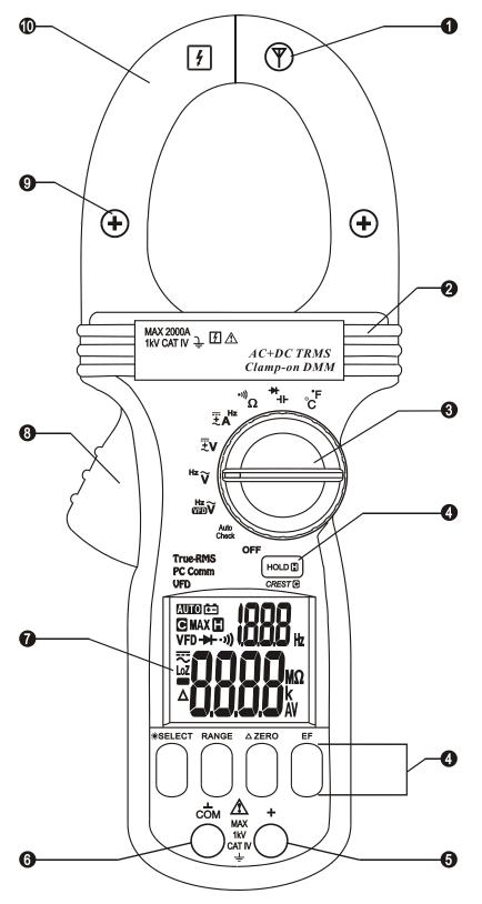
1) Antenna for Non-Contact EF-Detection
