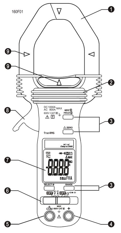
1) Hall-effect Clamp Jaw for AC & DC current electric field pick up
