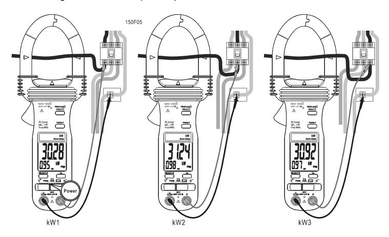
In both un-balanced and balanced load cases, 3-Phase 4-Wire (3 $\sim$ 4W) systems, measure the phase-to-neutral powers kW<sub>1</sub>, kW<sub>2</sub> and kW<sub>3</sub> of each phase separately as illustrated. System (total) power kW<sub>Total</sub> is the summation of all three phase-to-neutral powers. That is:
